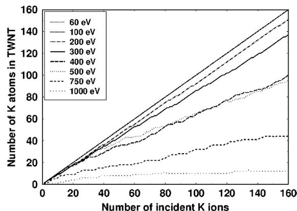
Fig. 5. Number of K atoms in a (5–10–15,0) TWNT as a function of the number of incident K ions. The data for 60 eV and 100 eV are identical and thus only the data for 100 eV can be seen from the figure.
