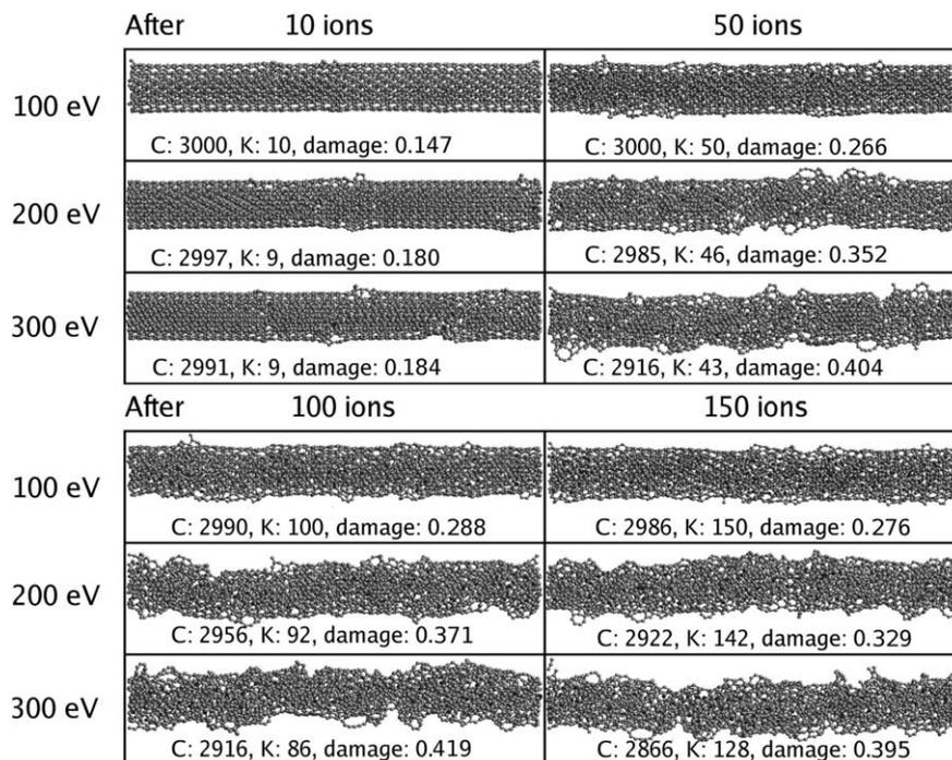
Fig. 10. A ball-and-stick picture series of a (5–10–15,0) TWNT irradiated with K using energies 100 eV, 200 eV and 300 eV. Shown pictures are after 10, 50, 100 and 150 K ions. Nearly all visible atoms are carbon. K atoms are a bit darker, but they can barely be seen. Below each picture the number of C and K atoms in the structure are written along with the damage ratio.
