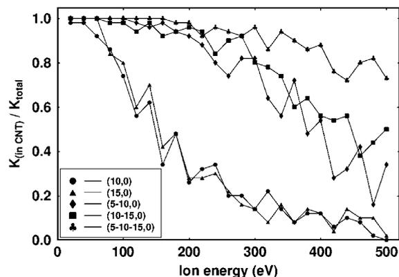
Fig. 4. Probability of K atom to penetrate the outermost wall of CNT and to stay within the CNT volume as a function of the initial ion energy for all simulated CNTs.
