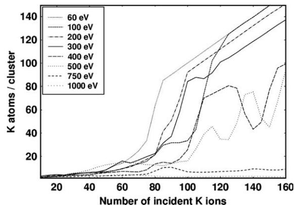
Fig. 6. Average cluster size in a (5–10–15,0) TWNT as a function of the number of incident K ions. To clarify the data, we calculated the average of nine surrounding data points for the same energy into a single point in the graph. The large jumps in the graphs are due to large clusters first joining and then parting again.
