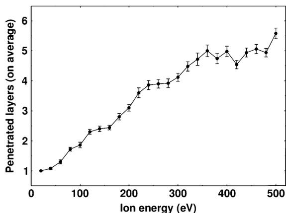
Fig. 1. The averaged number of penetrated graphitic layers as a function of the ion energy.
