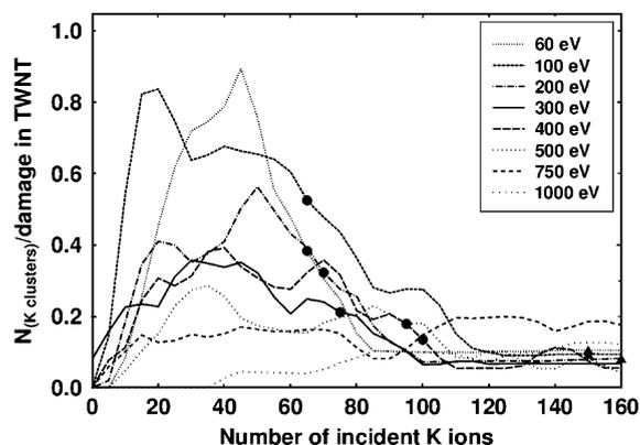
Fig. 9. Clusters/damage ratio of a (5–10–15,0) TWNT as a function of the number of incident K ions. Every data point in the figure is averaged from nine surrounding data points for the same energy to clarify the data. Points where the structures have a stoichiometry  $KC_{48}/K_3C_{60}$  are marked with a circle/triangle for each simulation energy. Some of the values did not fit in the  $x$ -axis range chosen for the figure.
