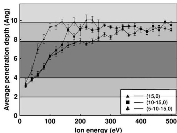
Fig. 3. Averaged penetration depth of K as a function of the ion energy. The (15,0) SWNT is shown with the lightest, the (10,0) SWNT with darker and the (5,0) SWNT with the darkest grey. The (10–15,0) DWNT contains both SWNTs (10,0) and (15,0) within each other and the (5–10–15) TWNT contains all of them.
